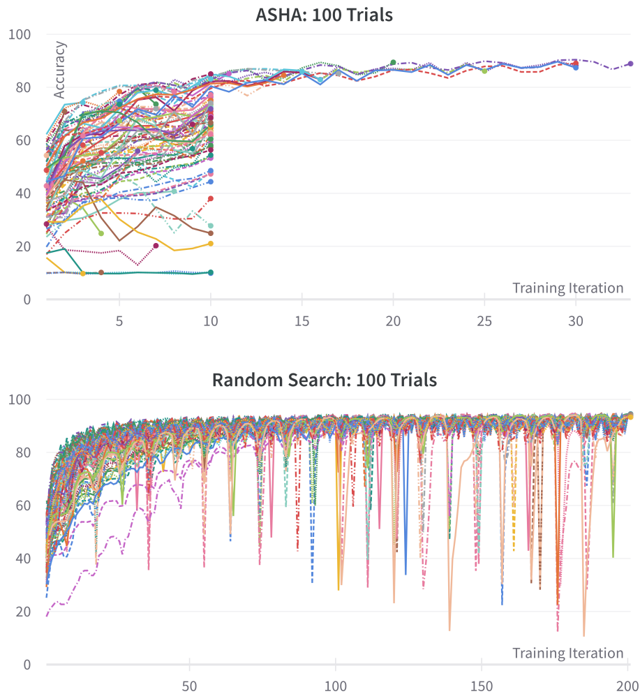
Figure 7: Comparison of the accuracy over the number of epochs (training iteration) for the ASHA algorithm (top), where under-performing trials are stopped early, to a simple random search algorithm (bottom), where every sampled configuration is fully trained on cifar-10. In the ASHA case, one training iteration corresponds to six training iterations in the random search case. 100 trials are evaluated in parallel on the JURECA-DC-GPU partition.
